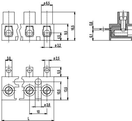
The screw/solder terminal strip 321-LFS in 10 mm pitch was designed for larger cross-sections than version 302-LF-DS. It is available with 1 to 12 poles.
